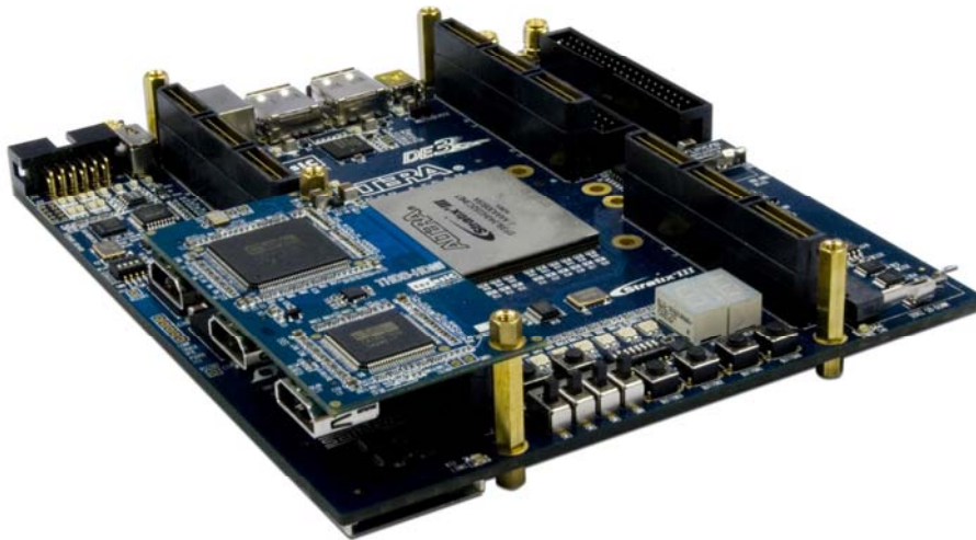
Figure 1.2 Connect HDMI daughter board to DE3 board
