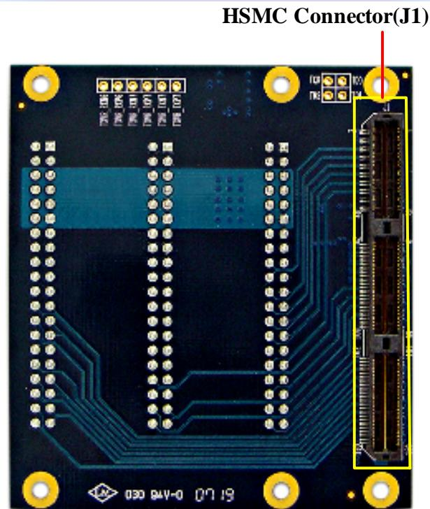
Figure 2.2 The TDRB-H2G board back side – HSMC connector view
