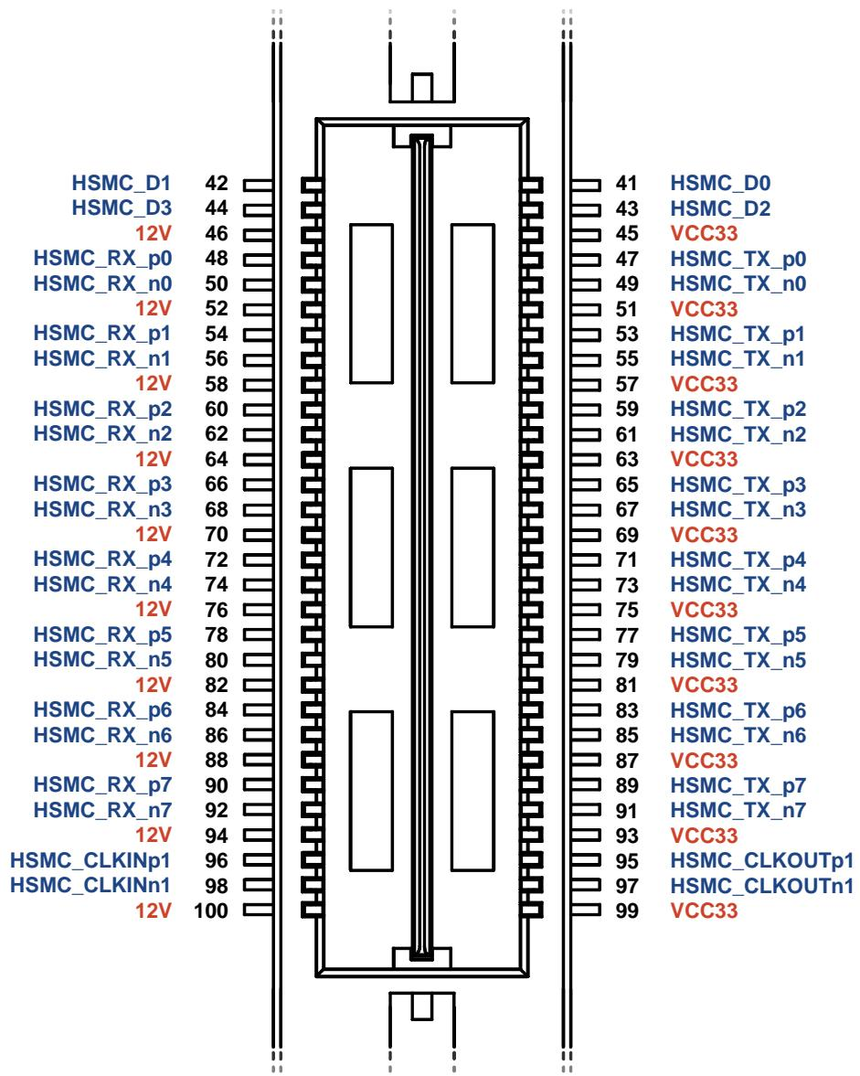
Figure 3.2 The pin-outs of Bank 2 on the HSMC connector
