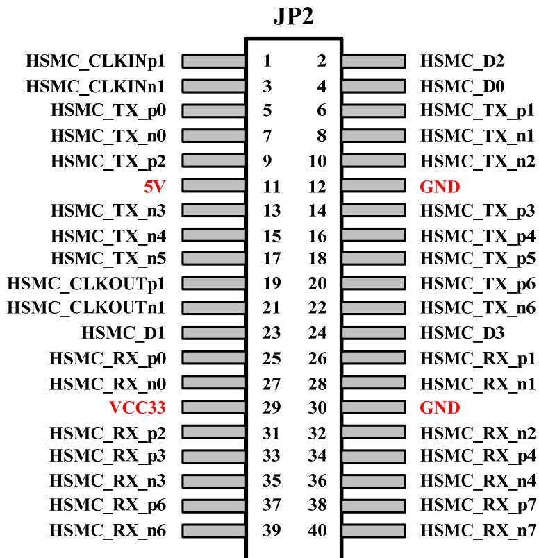
Figure 3.5 The pin-outs of the expansion prototype connector JP2
