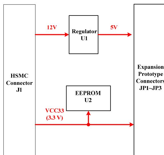
Figure 3.7 THDB-H2G board power distribution diagram.
