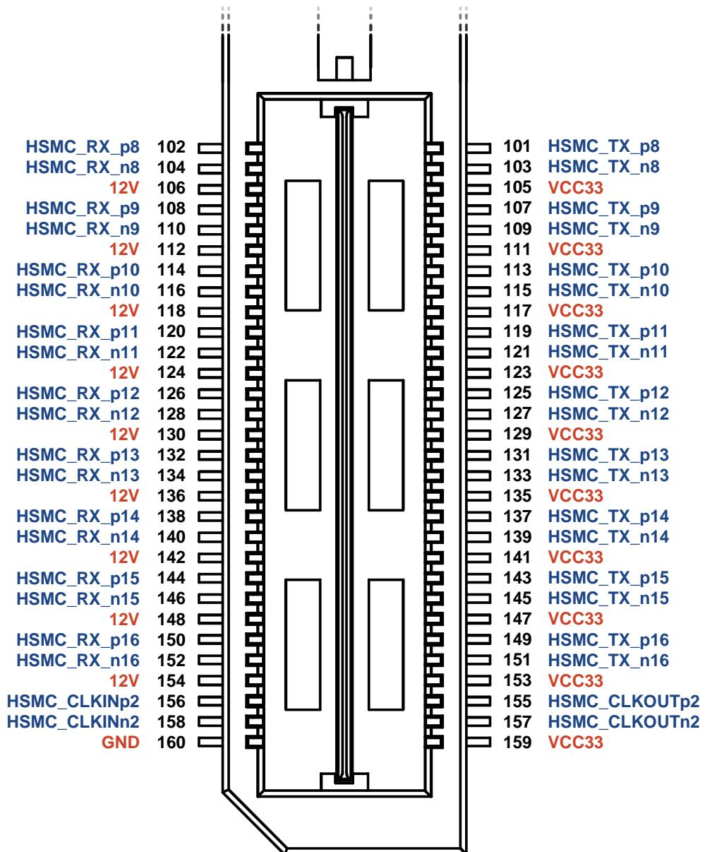
Figure 3.3 The pin-outs of Bank 3 on the HSMC connector.
