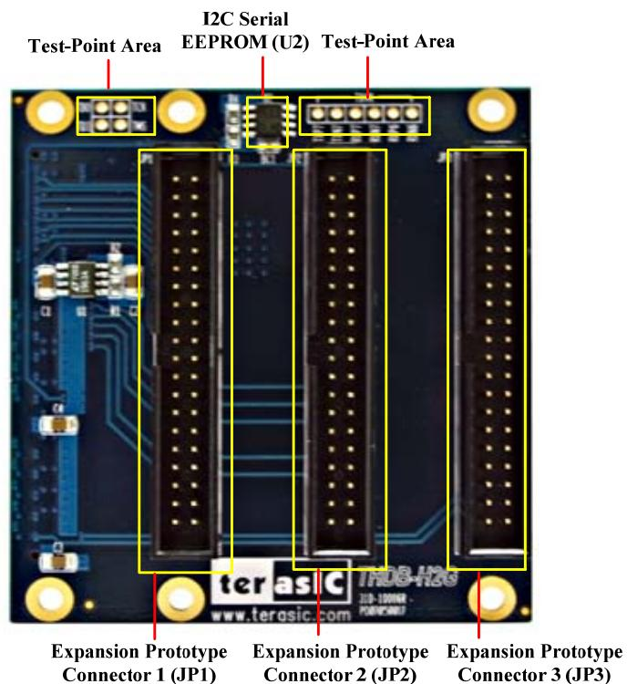
Figure 2.1 The TDRB-H2G board PCB and component diagram
