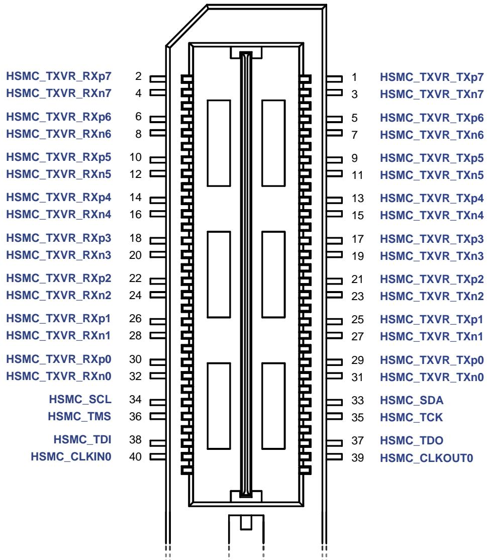
Figure 3.1 The pin-outs of Bank 1 on the HSMC connector.
