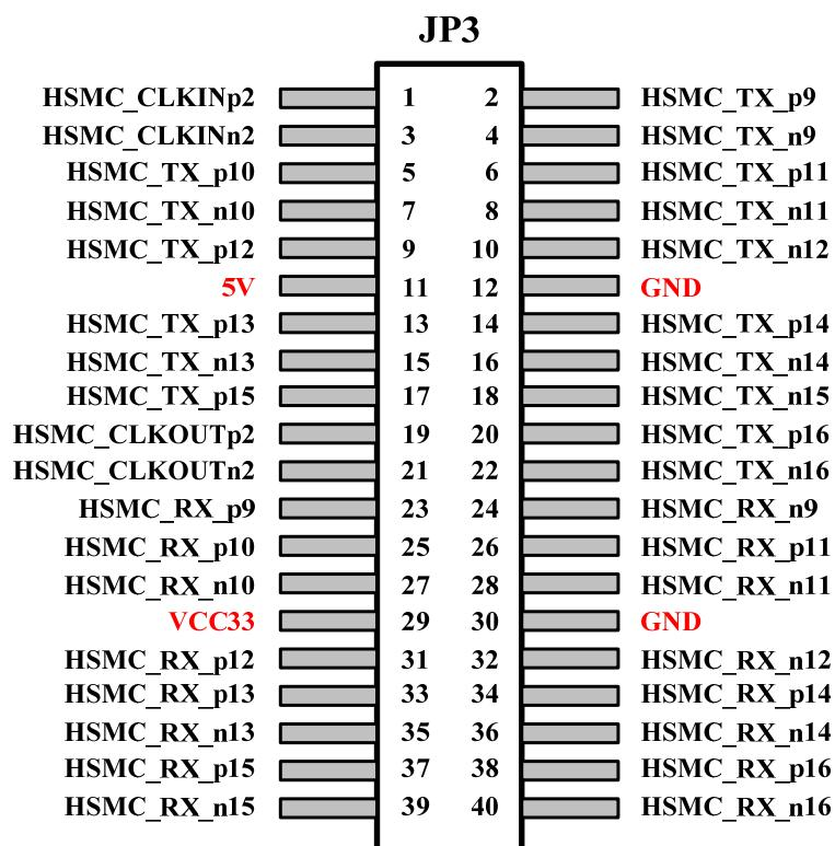
Figure 3.6 The pin-outs of the expansion prototype connector JP3
