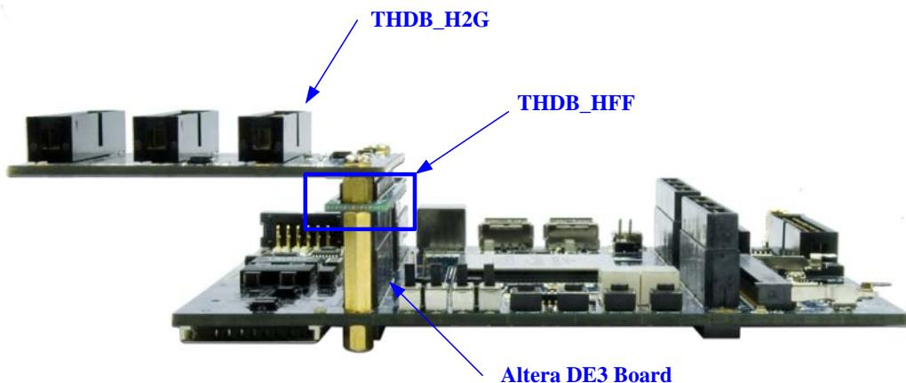
Figure 4.2 Connecting the THDB-H2G board to the Altera DE3 board
