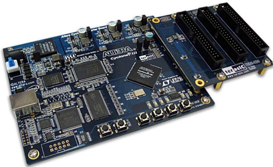
Figure 4.1 Connecting the THDB-H2G board to the Cyclone III starter board
