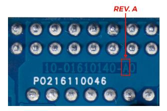
**3.** For revision B and B2, please check the serial number on the board, as shown below. If the number is "17040025-XXXX", the board is revision B2. Otherwise the board is revision B.
