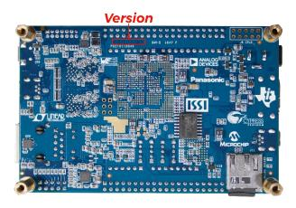
2. If there is an "A" printed at the specified location shown below, it refers to revision A. If the character is "B", it indicates the revision is B or B2. For revision C, the letter printed would be C.
